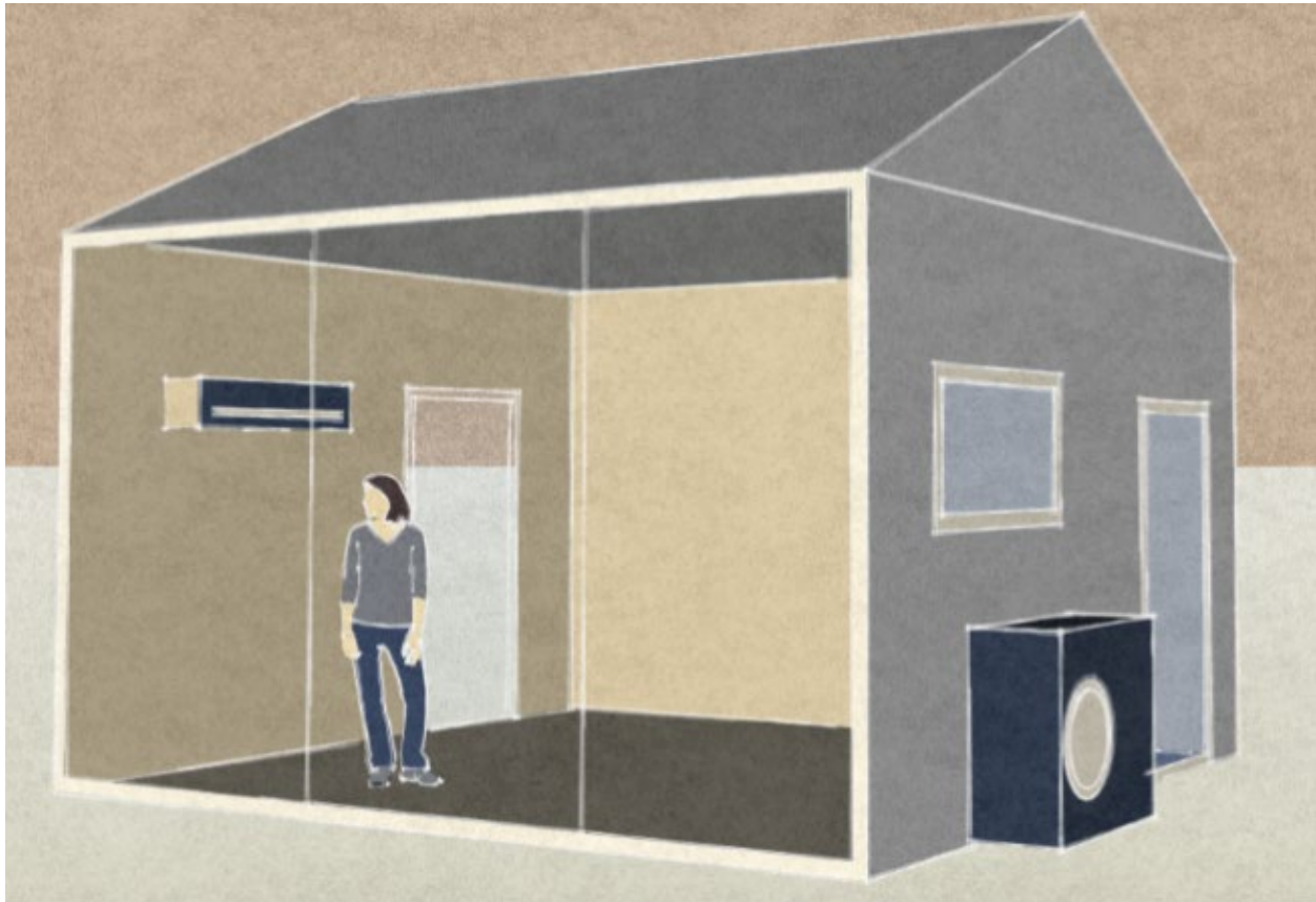
Figure 29: scale illustration of split air to air heat pump with external unit ( right ) connected to internal fan coil unit ( top left ). No radiators and no hot water.
