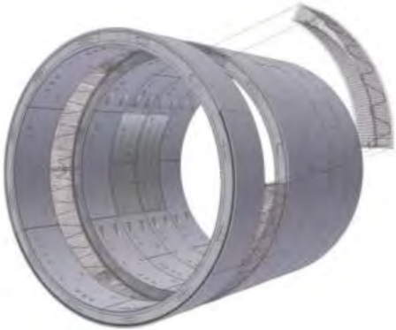
Geothermal Tunnel Lining
