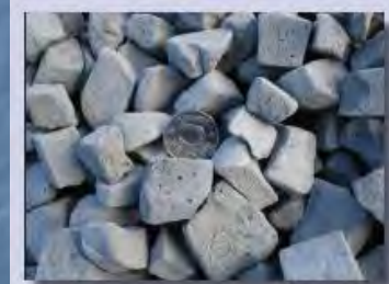
The insulation consists of 0.4 m expanded glass (foam glass)
