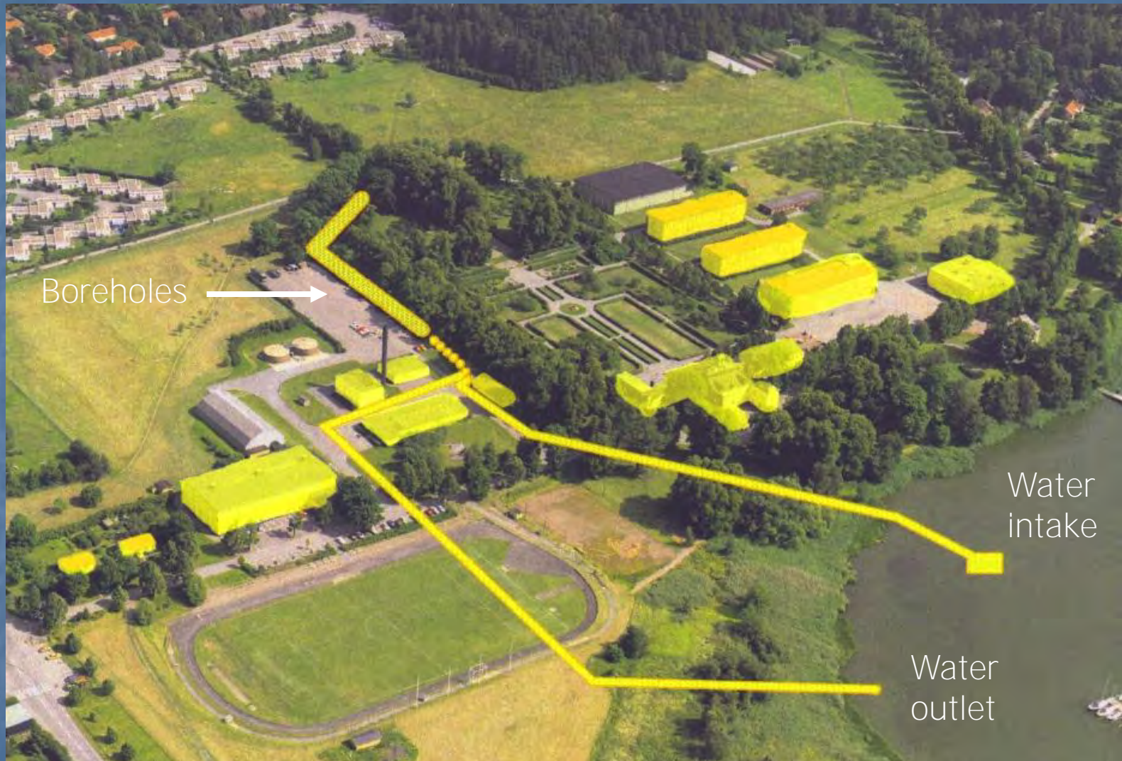
Hybrid system - Boreholes with summer recharge from lake
