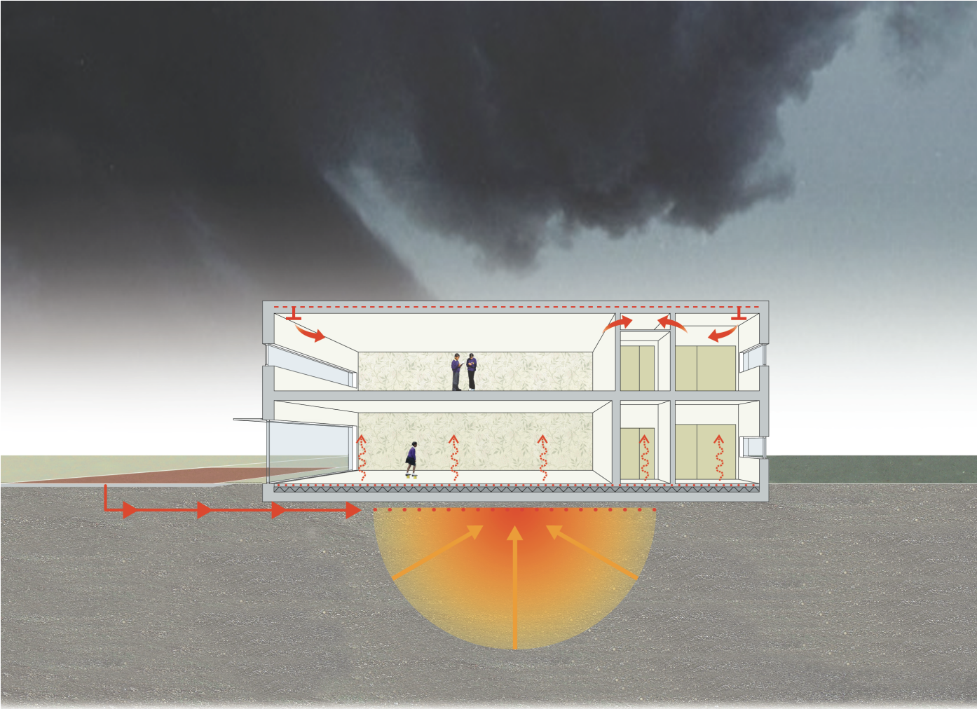
In winter heat is transferred from the ThermalBank up to the building - without burning fossil fuels
