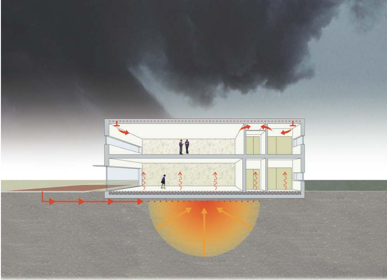
During the winter the heat is transferred from the ThermalBank up to the building - without burning fossil fuels
