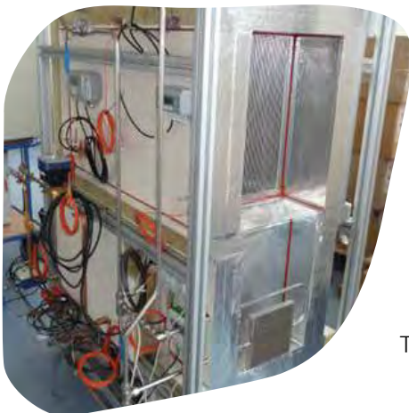
Open sorption storage system
