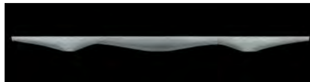
Figure 2.18: Concrete beam made with fabric formwork
